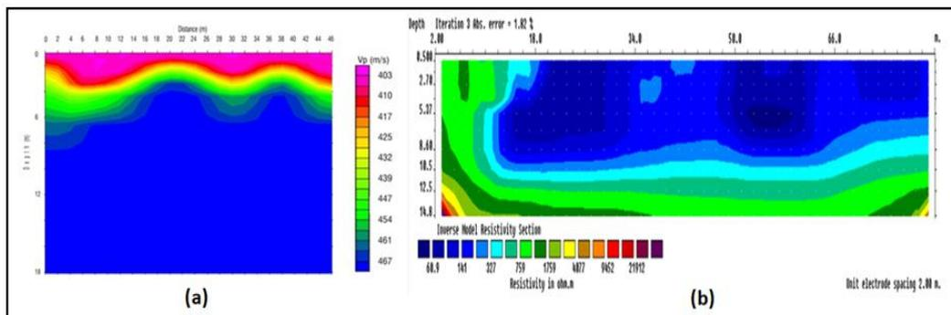
Figure 3: 2D P-wave velocity and Electrical Resistivity Model Tomograms at a common survey line at Uruagu-Nnewi Site
