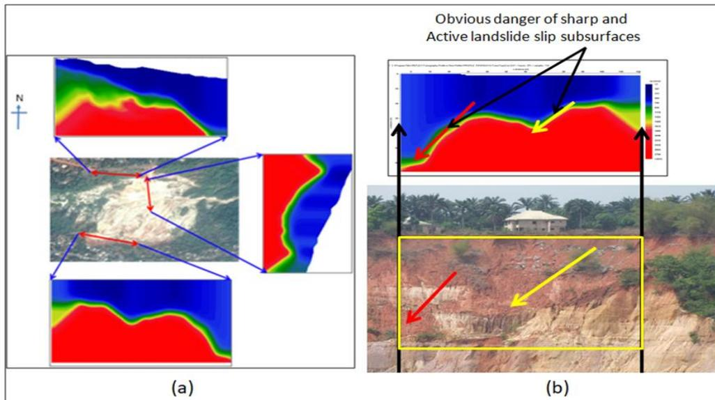
Figure 4: 2D P-wave velocity Model of seismic Refraction Tomograms at three profile lines surveyed at Nanka-Oko Site (a) showing the orientation of the survey lines and the tomogram and (b) showing the danger of sharp and active landslide slip surfaces
