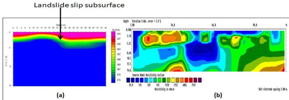
Figure 2: 2D P-wave velocity and Electrical Resistivity Model Tomograms at a common survey line at Uruagu-Nnewi Site
